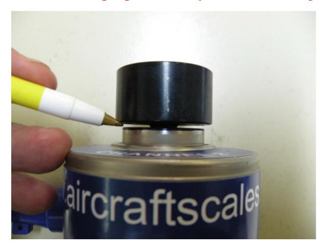
Below is a picture of an improper install, note that the adapter is not all the way bottomed and there is an air gap. Cells with air gap will read incorrectly, can be damaged and may cause damage to the aircraft.
