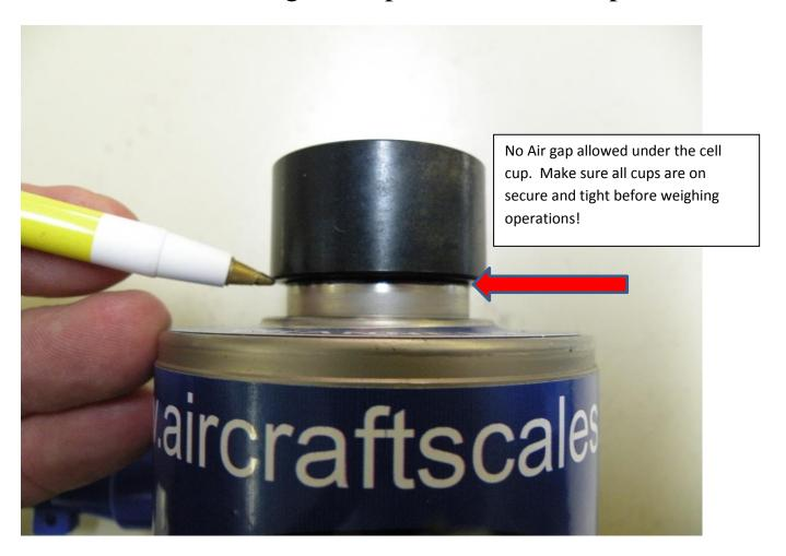
Note: It is very important that the cell top jack pad adapters are screwed in all the way as shown with no air gap, adapter <u>must</u> bottom on the cell top.
