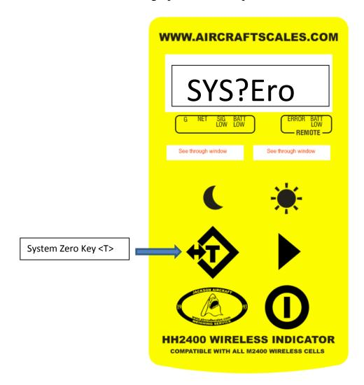
On power up the unit is set to default and read the total weight of all cells. In this mode, pressing the tare key and holding it will force a System Zero.
